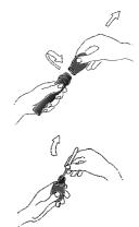
2. Pull out the foam pop shield, if necessary use tweezers.
